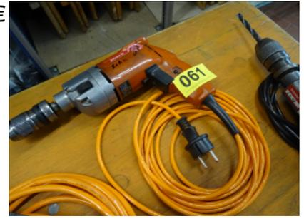
**62 Bohrmaschine KINETIK**
